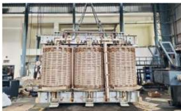
Coil Assembly of 20MVA Power Transformer
